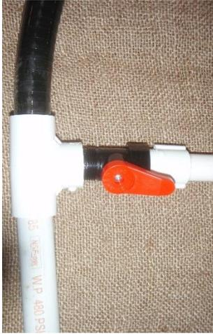
The purpose of the (black) flexible pipe is to make it easy to route the water supply out of the reservoir into the main 1" supply line. You can attach the flexible pipe to the side of the wooden frame as shown in the pictures in that document.
