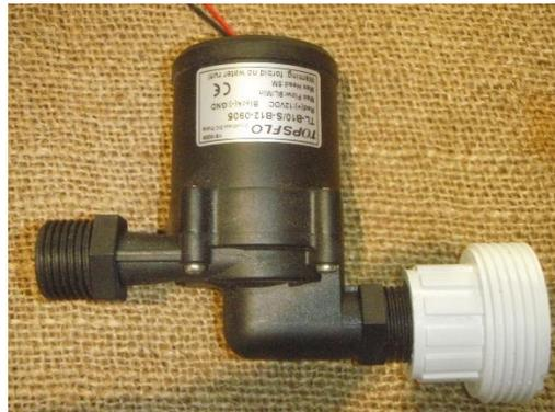
On the other side of the union, attach the  $\frac{1}{2}$ " threaded to  $\frac{3}{4}$ " slip male adapter.
